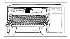
**To install a new filter,** remove plastic and other outer wrapping from the new filter. Insert filter into top opening of oven as shown. It will rest at an angle on two side support tabs and in front of right rear tab. Replace grill and secure with 2 screws.
